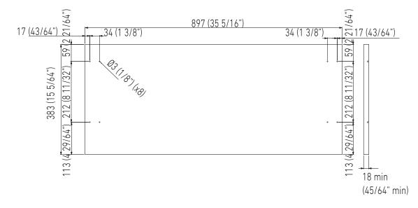
Panels with thickness ranging between 18 mm and mm. Panels with weight max of 12 kg. Provide installation of decorative panels during installation of the unit.
