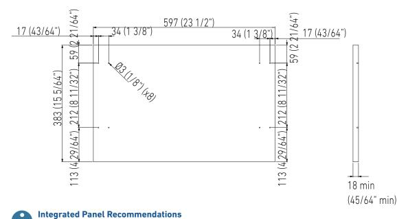
Panels with thickness ranging between 18 mm and mm. Panels with weight max of 8 kg. Provide installation of decorative panels during installation of the unit.
